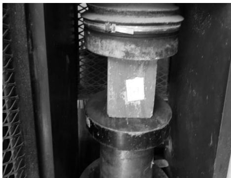
Figure 1: Compressive Strength Testing for Cube
